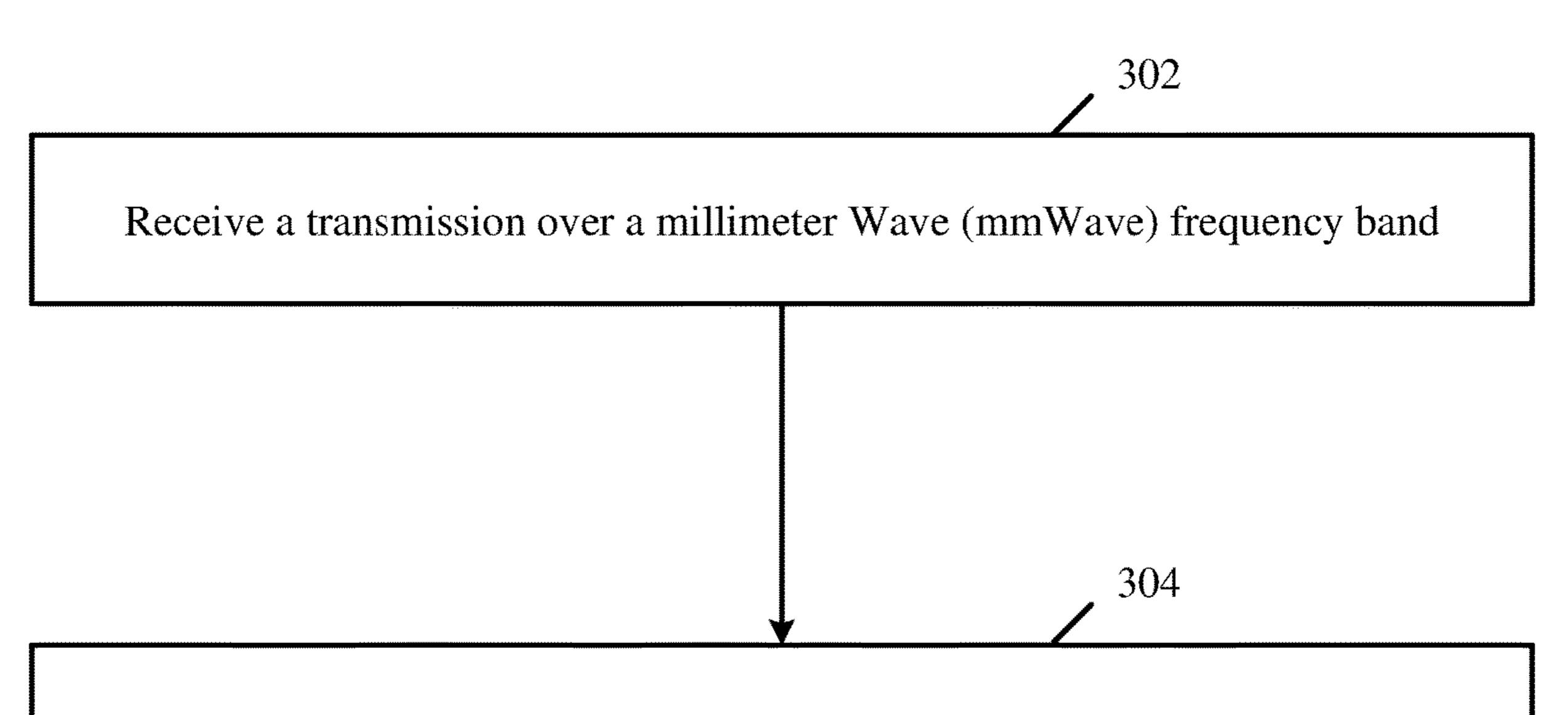
Decode a plurality of data bits from the transmission according to a Low-Density Parity-Check (LDPC) code having an encoding rate of 7/8 and a codeword length of 1248 bits
