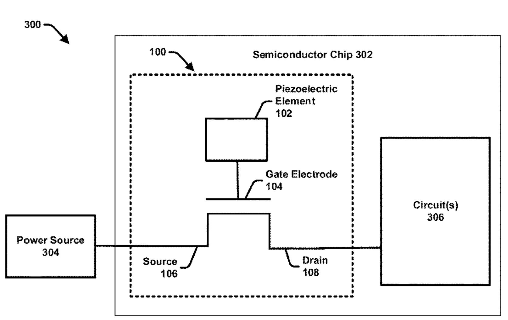
mechanical force, thereby causing the pass transistor to be in an on-state. In one implementation, the two or more electrical components comprise a circuit and a power source. In another implementation, the two or more electrical components comprise two circuits.
