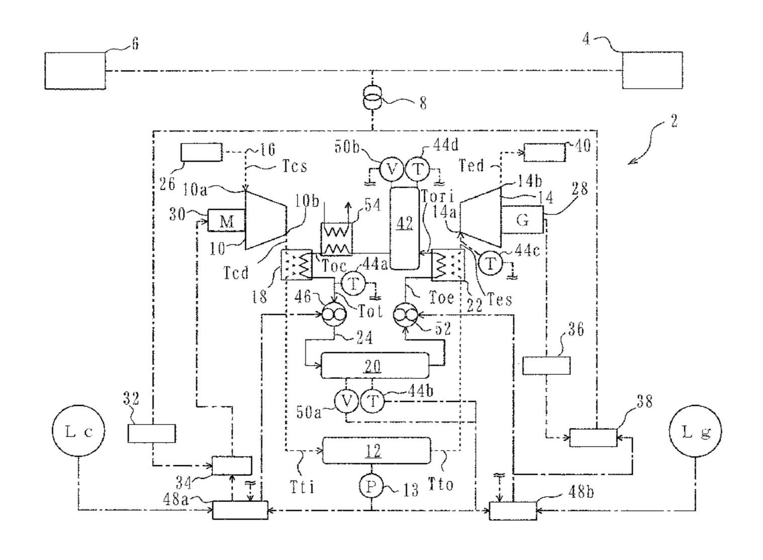
pump adjusts an amount of the heat medium to be supplied to the first heat exchanger. A control device controls the first pump to adjust the amount of heat medium to be supplied to the first heat exchanger so as to maintain the heat medium, which is stored in the heat medium tank, at a predetermined first temperature.
