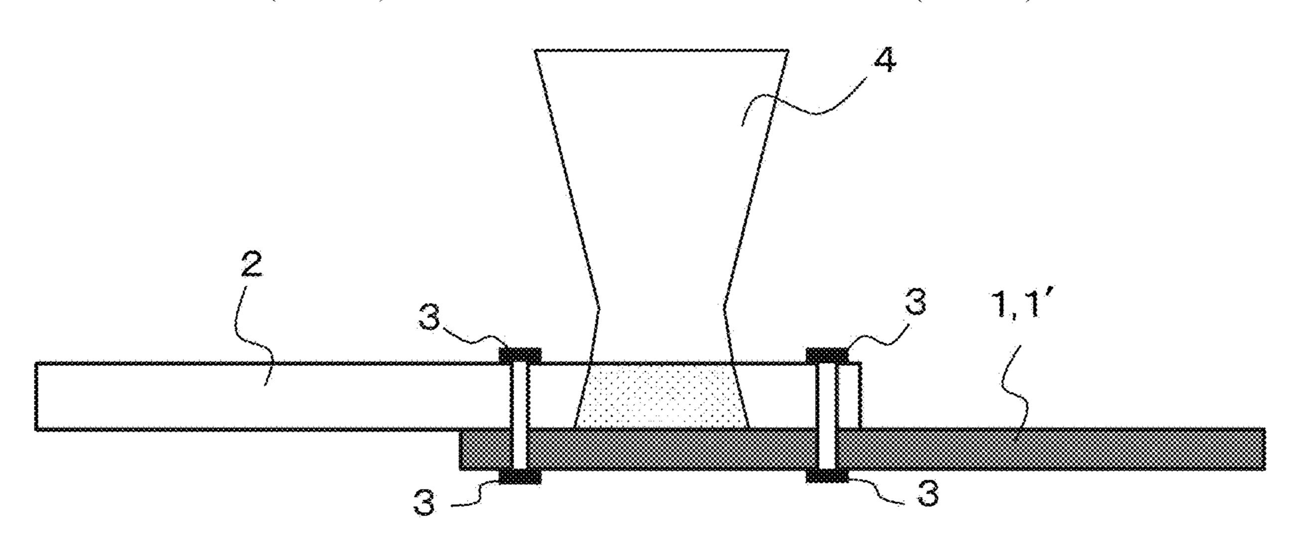
laser beam from the plastic member side through the glass at a joining location where the metal and the plastic member are overlaid to join them by a joining speed of 0.5 m to 5.0 m/min.
