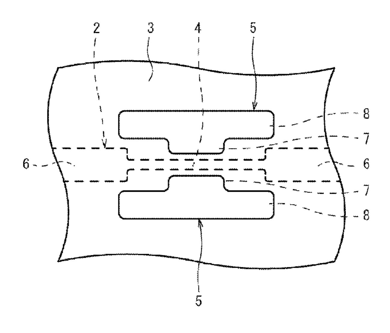
side of the base film. The conductive pattern forms part of a circuit and includes at least one fuse portion having a cross section smaller than the other part. The flexible printed circuit board includes at least one opening passing through front and rear surfaces on at least one of the right and left sides of the fuse portion in a two-dimensional view.
