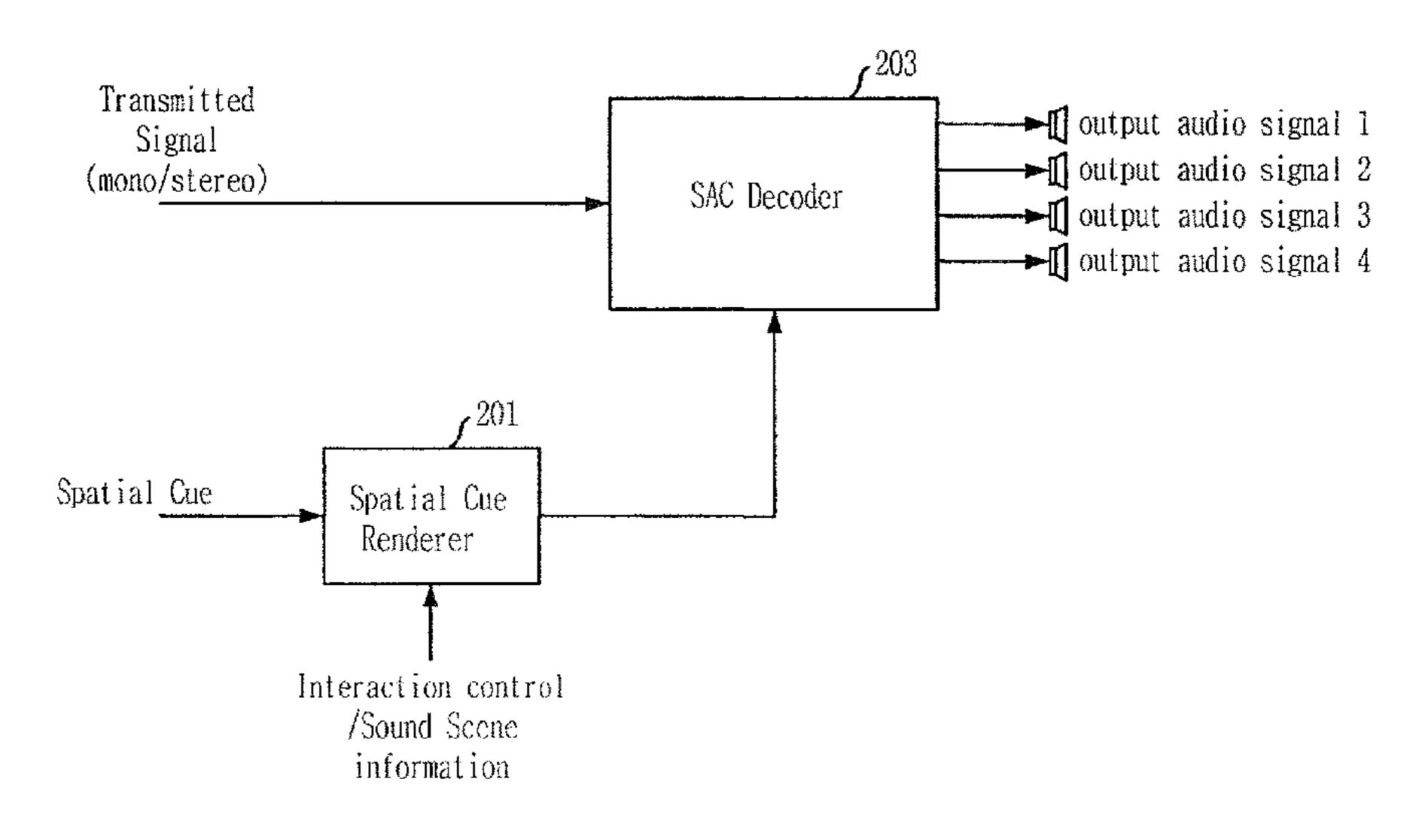
based on spatial cues in a process of decoding the multiobject or multi-channel audio signals. To achieve the purpose, the method suggested in the research controls rendering in a spatial cue domain in the process of decoding the multi-object or multi-channel audio signals.
