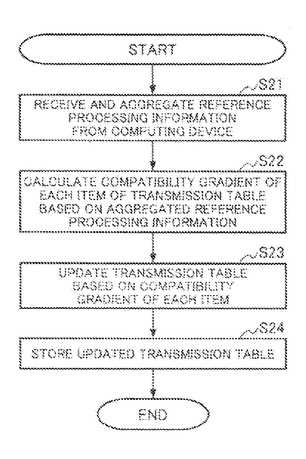
reference processing information, and a transmission table update unit that updates the transmission table based on the calculated compatibility.
