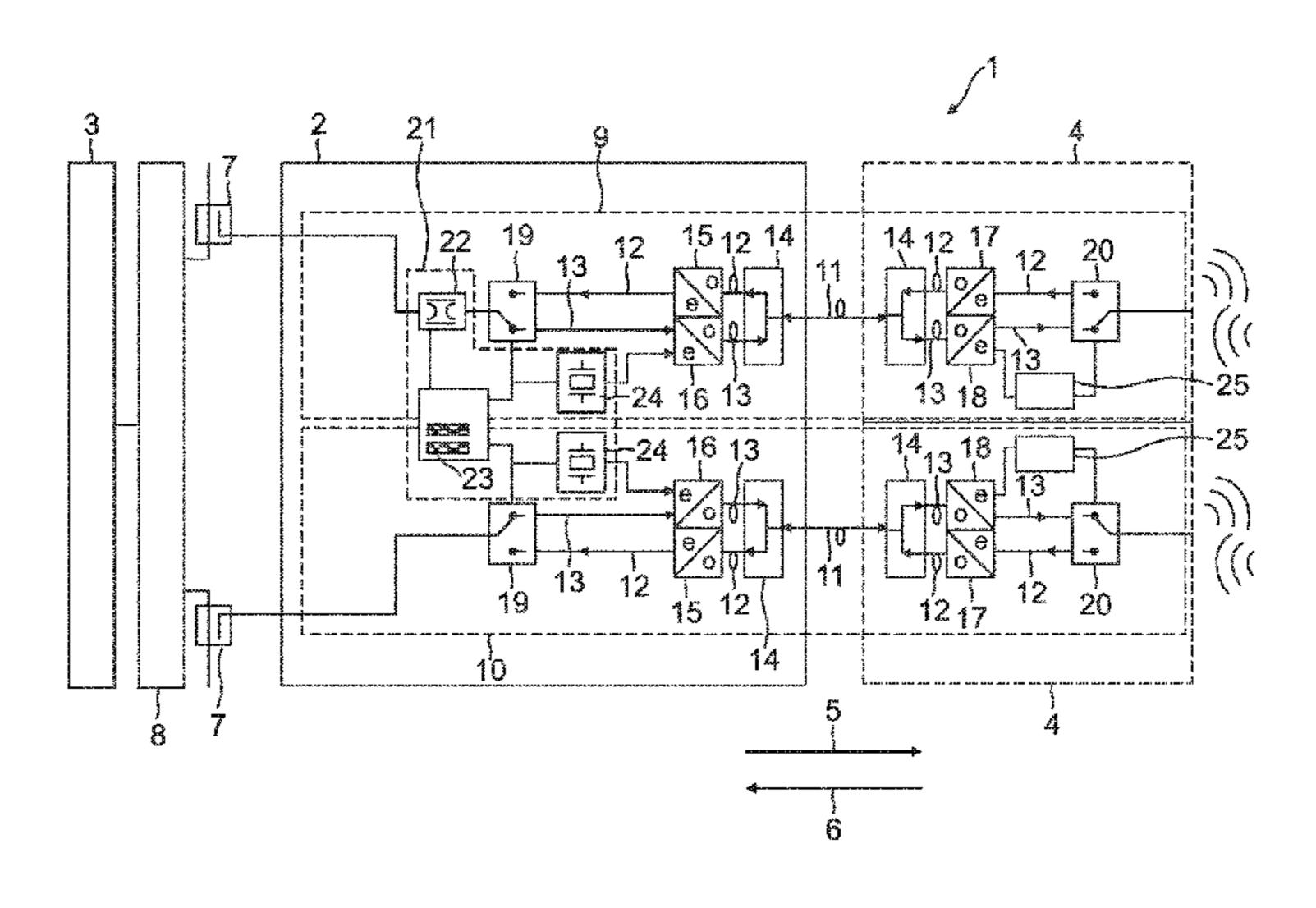
signals; a synchronizing unit is configured to receive via the downlink signal path a clock signal from the downlink communication signals, wherein the synchronizing unit supplies a control signal to the switch corresponding to the clock signal; wherein the switch swaps the direction of signal transmissions within the master unit between the uplink communication signals and the downlink communication signals in response to the control signal.
