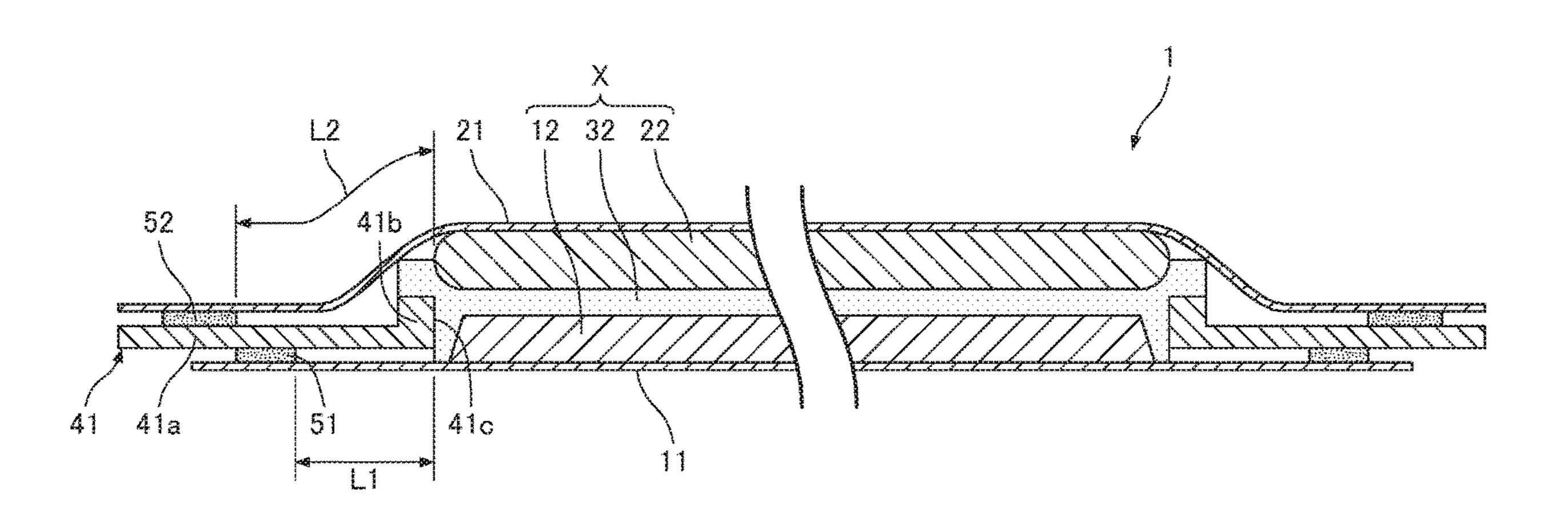
positive electrode layer from the negative electrode layer. In the insulating member, a contact inner edge portion contacted with the laminate is thicker than a plate-shaped portion on the outer side.
