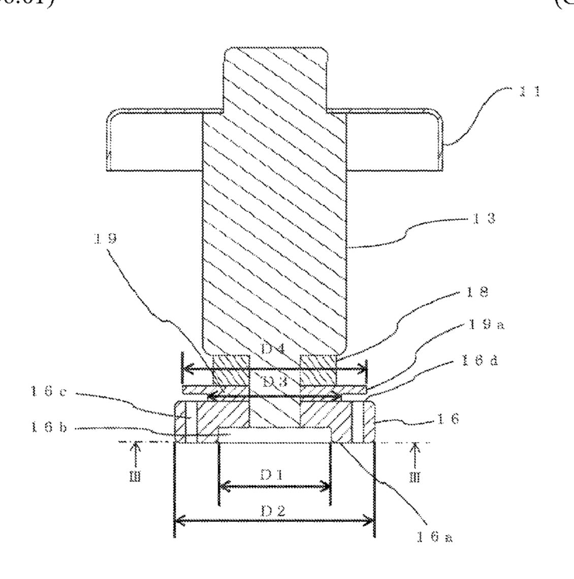
fixed side contact; and a movable side reinforcement plate which is arranged between the movable side electrode rod and the movable side contact, and whose rim portion has a step portion to be arranged apart from the back of the movable side contact.
