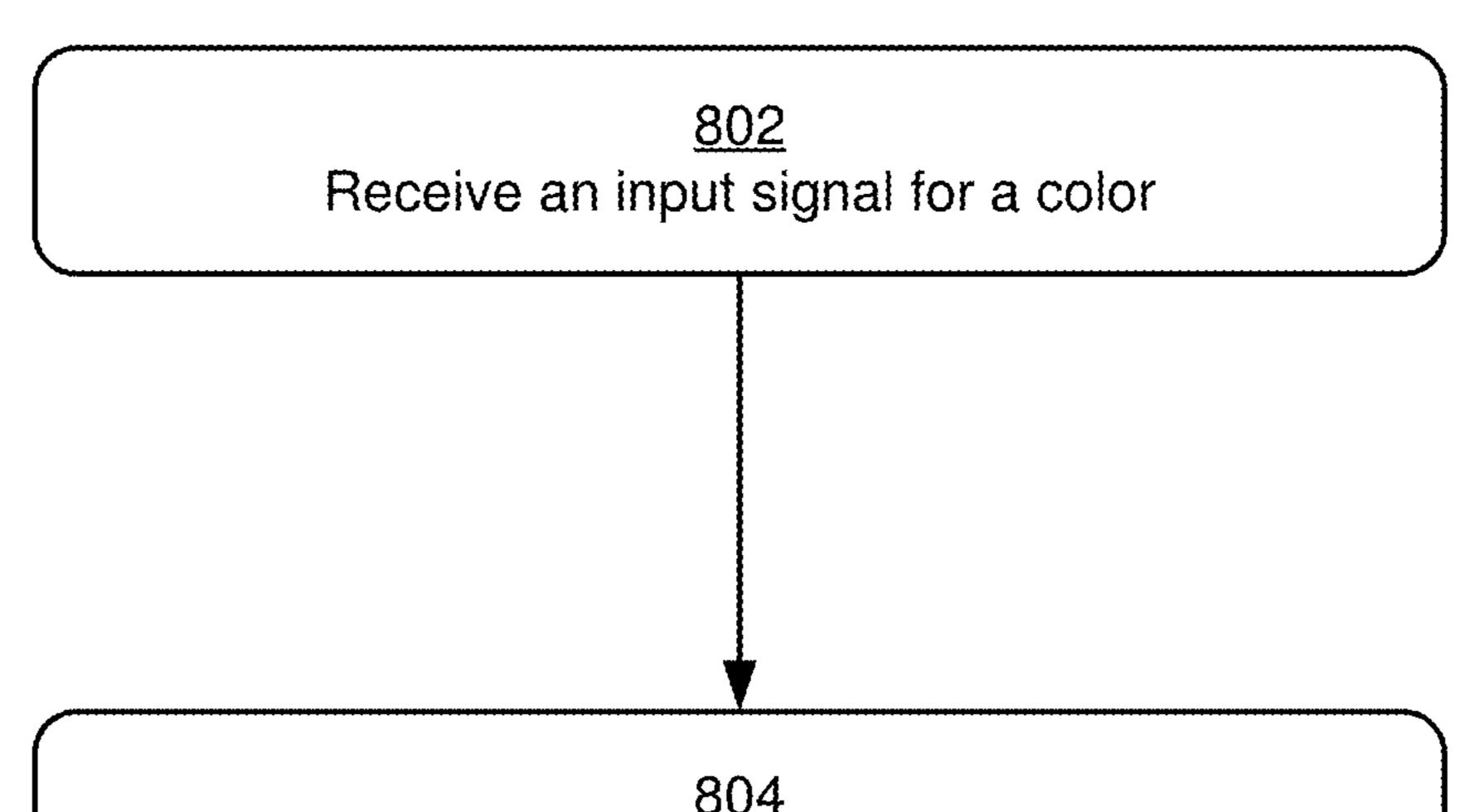
Apply a voltage to sub-pixels of the color such that a voltage across one or more additional sub-pixels of the color is proportional to a voltage across a first sub-pixel
