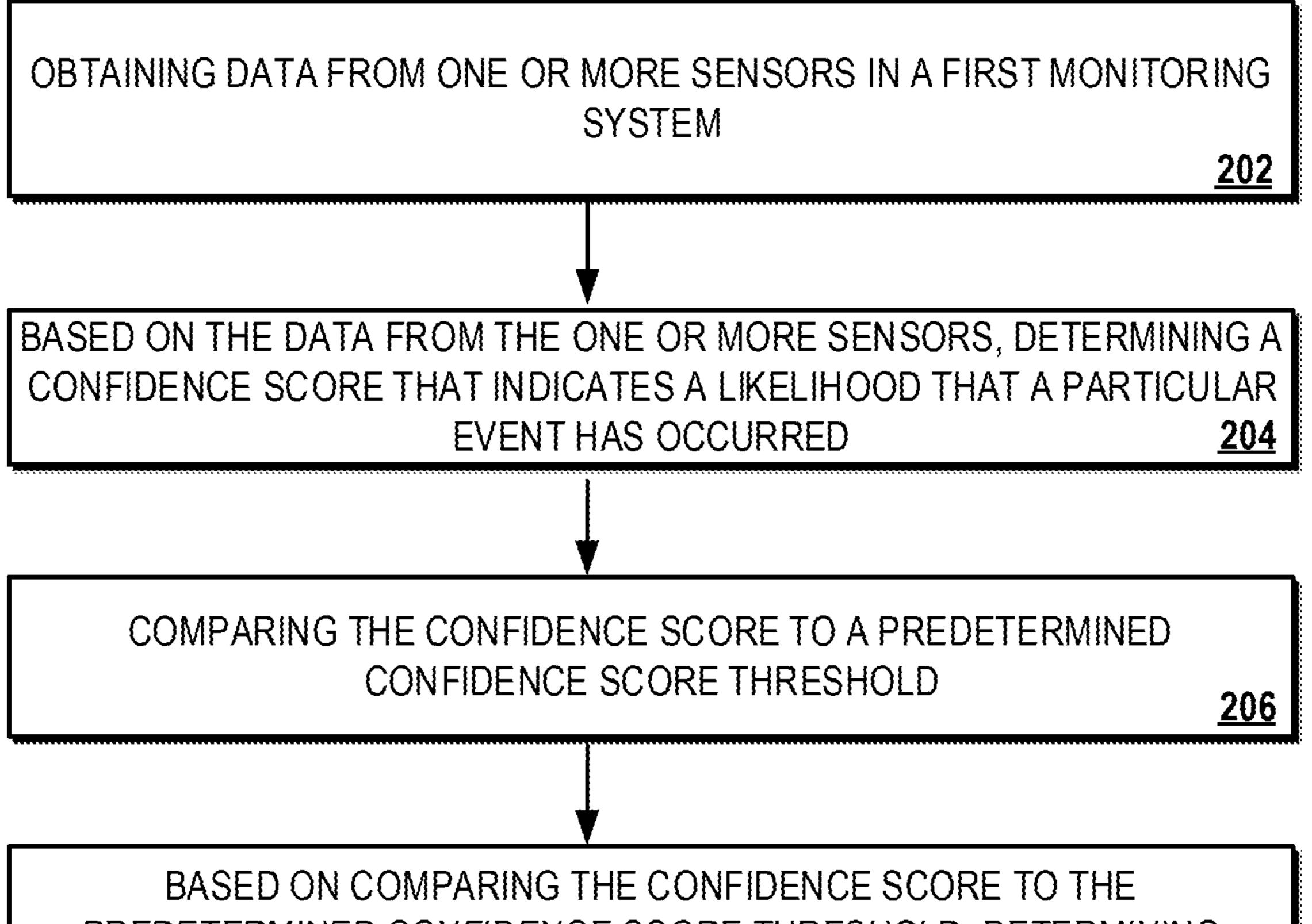
BASED ON COMPARING THE CONFIDENCE SCORE TO THE PREDETERMINED CONFIDENCE SCORE THRESHOLD, DETERMINING WHETHER TO PROVIDE, TO A SECOND MONITORING SYSTEM, DATA INDICATING THAT THE PARTICULAR EVENT HAS LIKELY OCCURRED 208
