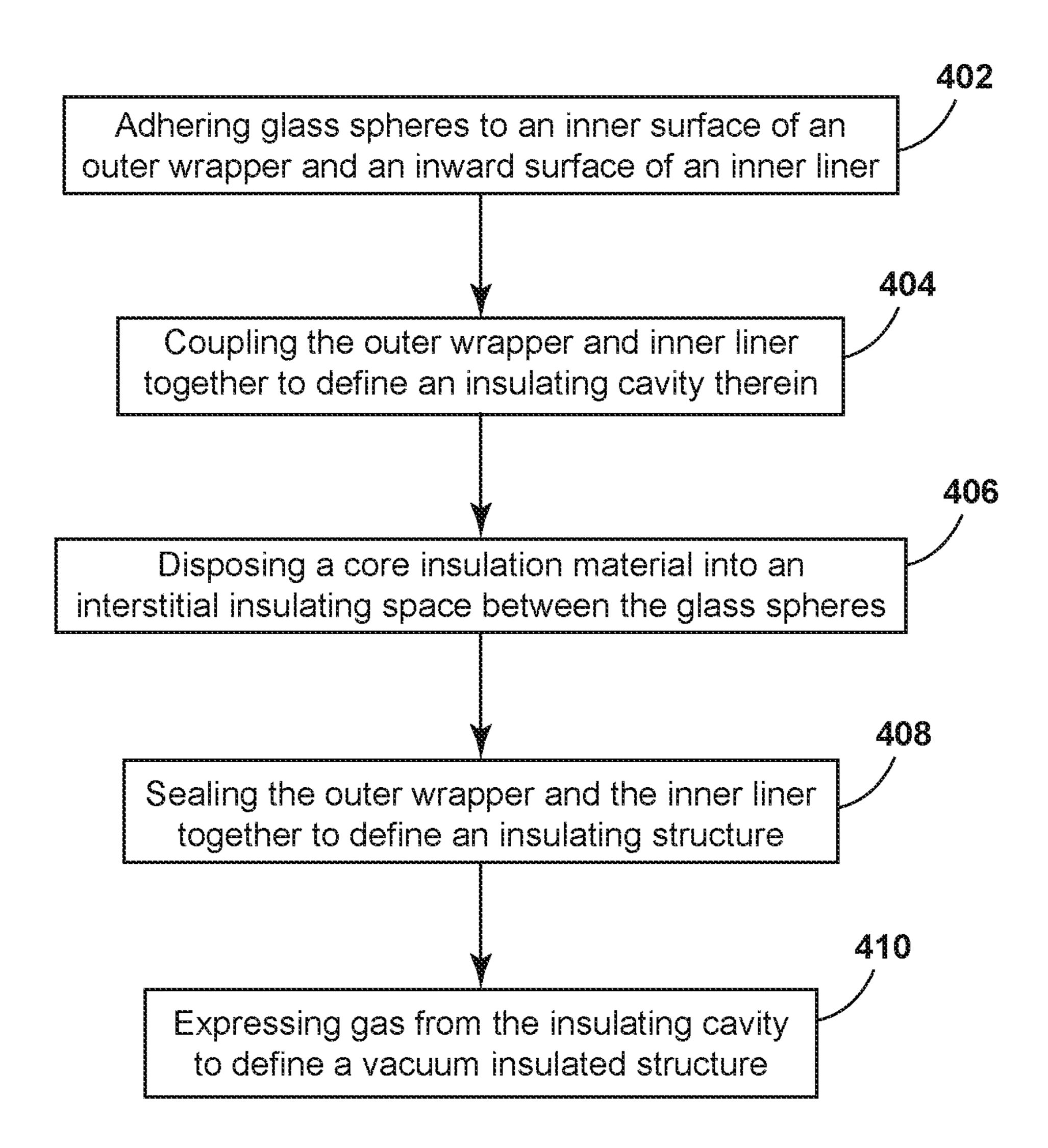
Method 500 for Forming a Structural Cabinet for an Appliance
