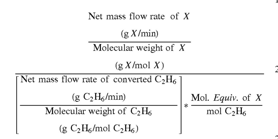
where X is the product that is being assessed, the net mass flow rate refers to flow in g/min for X or ethane entering the reactor minus the flow rate exiting the reactor, and molar equivalent (Mol. Equiv.) refers to the amount of X, in moles, 30 that reacts completely with one mole of ethane. Selectivity is referred to as a wt. % despite the fact the calculation results in converting wt % to a molar percentage because weight flow rate is the measurement that is used in the calculation.
