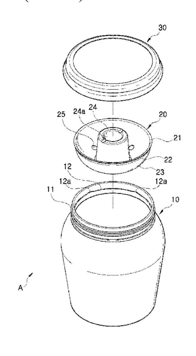
provided at the lower end of the vertical section and having a bottom surface part coming into contact with the surface of the fermented food.
