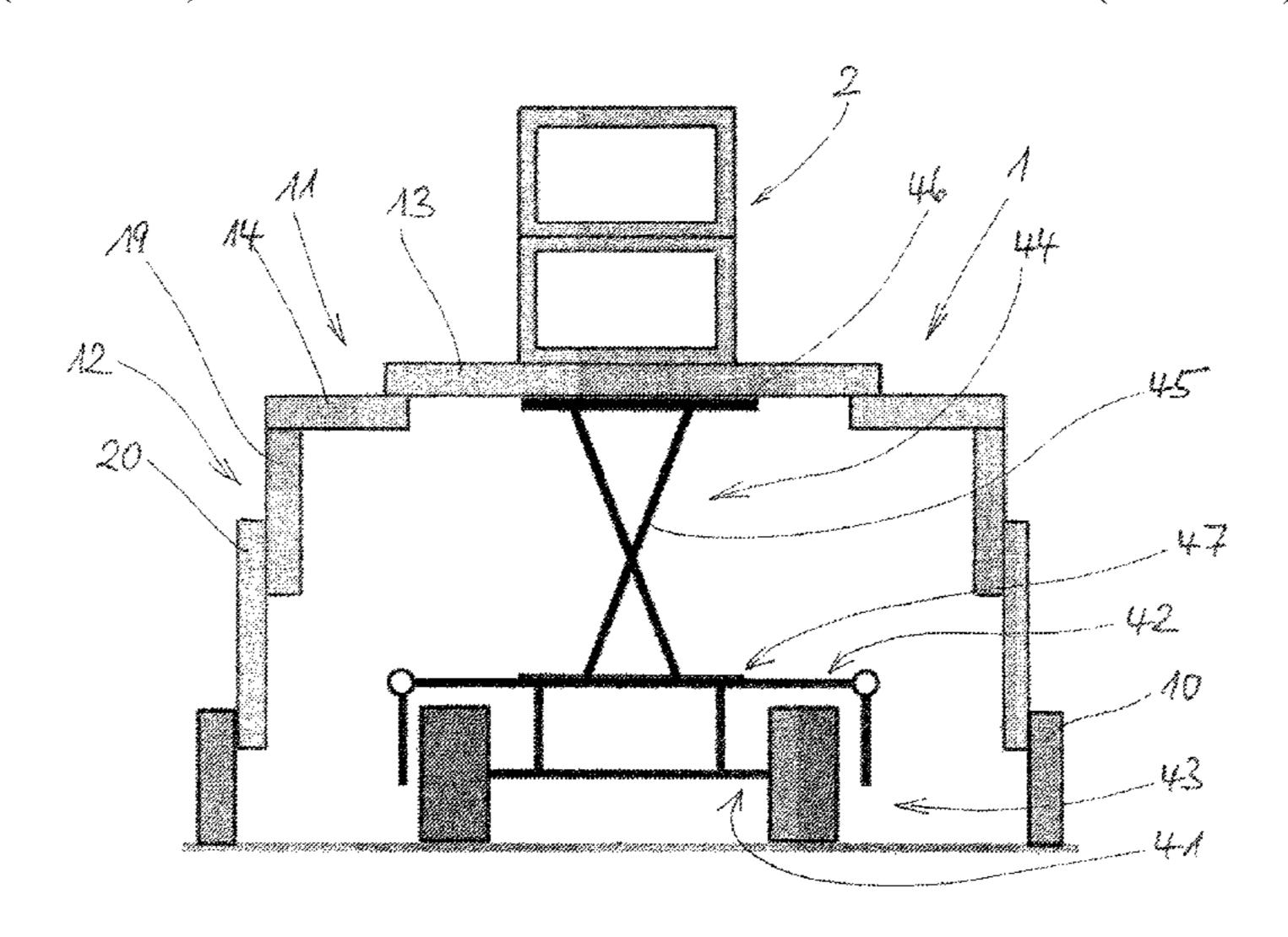
parts having primary parts connected to the associated end piece of the transverse structure and secondary parts, fixable thereon in various height positions and on which associated wheel-carrying units are disposed.
