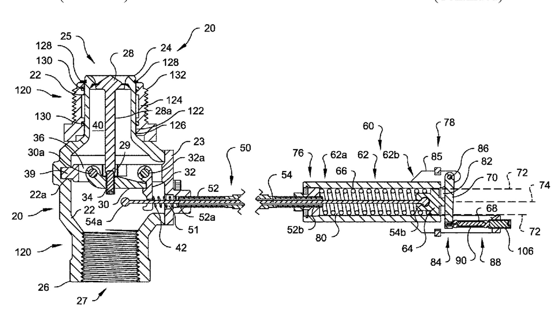
with the movable member. The flexible cable is moved with respect to the outer cable housing by movement of the movable member upon loss of structural integrity by the thermally responsive element.
