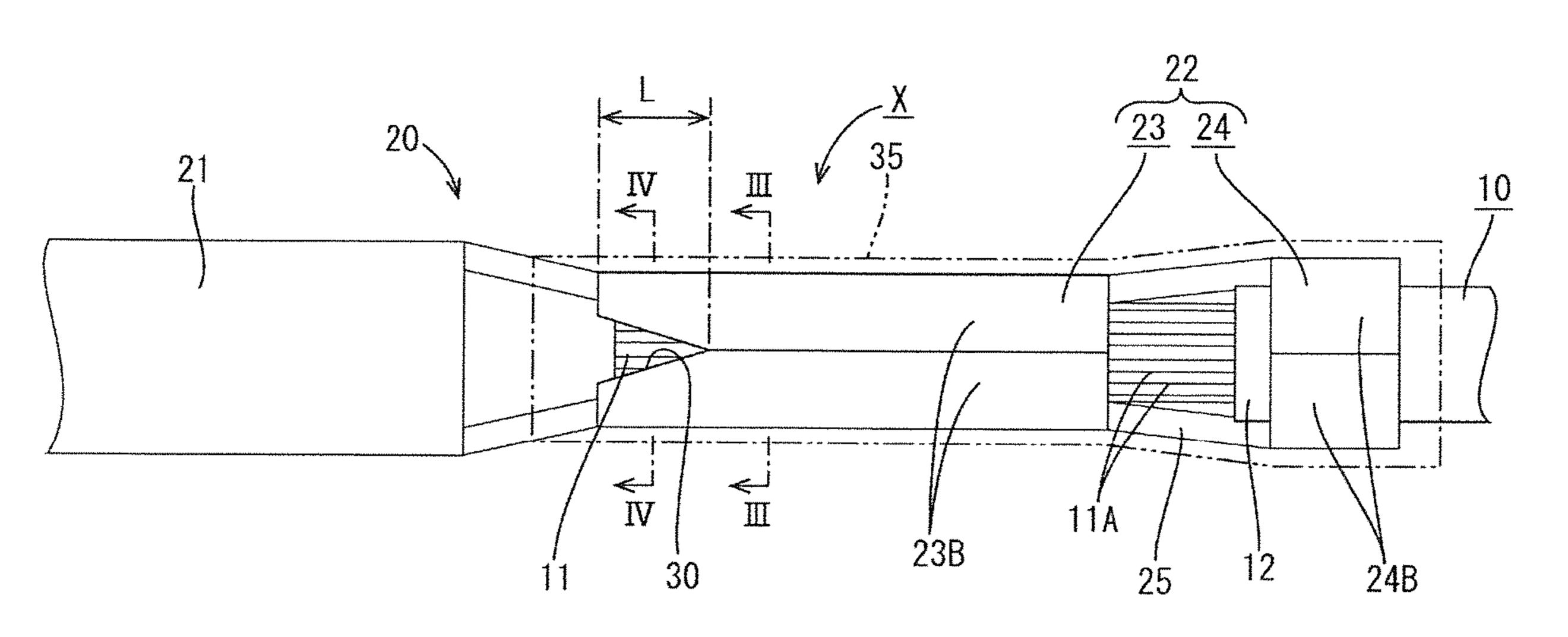
front of the crimped wire barrel (23) by widening an interval between corresponding butting parts of the barrel pieces (23B).
