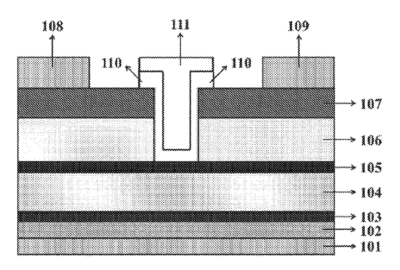
trode is provided on the top gate dielectric layer. The present disclosure provides a PMOS FET with better gate control functionality and a low interface density with the double-gate structure and interface control layer design, in order to meet the requirements of high-performance PMOS transistors.
