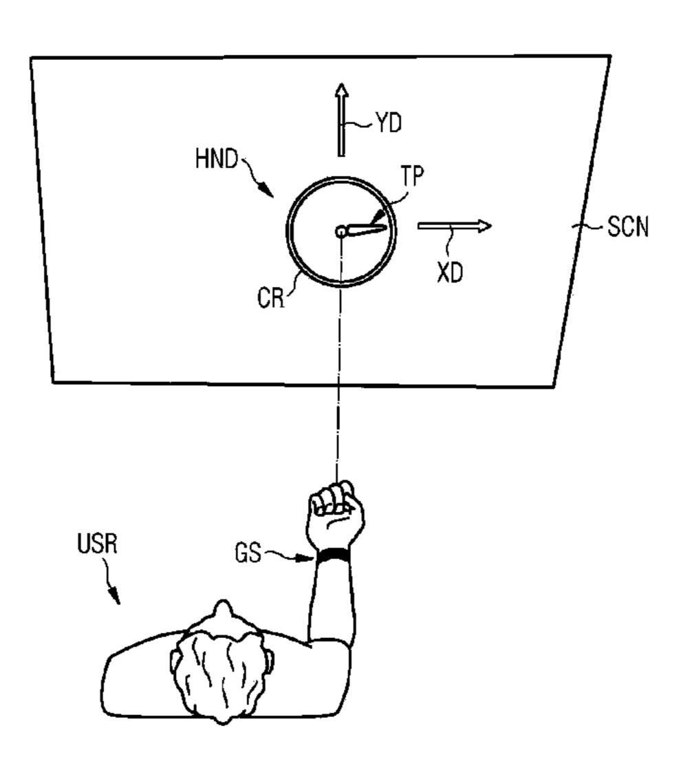
direction in which the forearm is pointing. In this manner, the operator may use shoulder rotation and elbow flexion to change the position of the forearm in order to change spatial parameters for a processing marker, while processing operations may be deactivated and/or activated by an independent rotation of the forearm.
