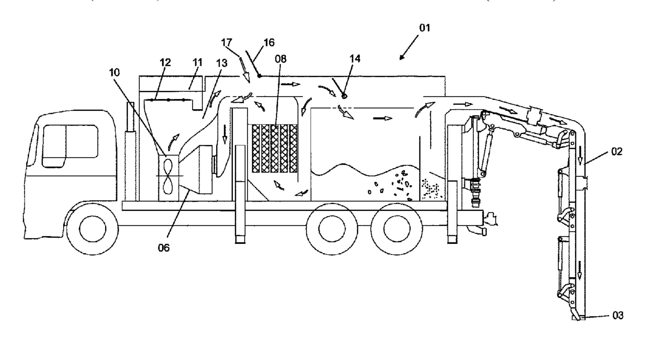
volume-controllable recirculation opening. A volume-controllable secondary air opening allows secondary air from the surroundings to be supplied to the suction side of the fan unit, downstream from the filter unit in the flow direction. The recirculation channel is fluidically coupleable to the suction hose to generate a positive pressure in the recirculation channel to blow out recirculation air through the suction hose.
