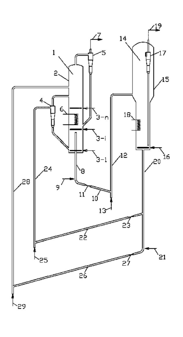
or more of the hydrocarbons with 5 or more carbons into a catalytic cracking lift pipe to perform a cracking reaction to generate a product containing propylene and C4 hydrocarbons, which is subsequently fed into a dilute phase zone of the fast fluidized-bed reactor. The method and device of the present invention improve the reaction rate of ethylene alkylation, and the unit volume production capacity of reactor is high.
