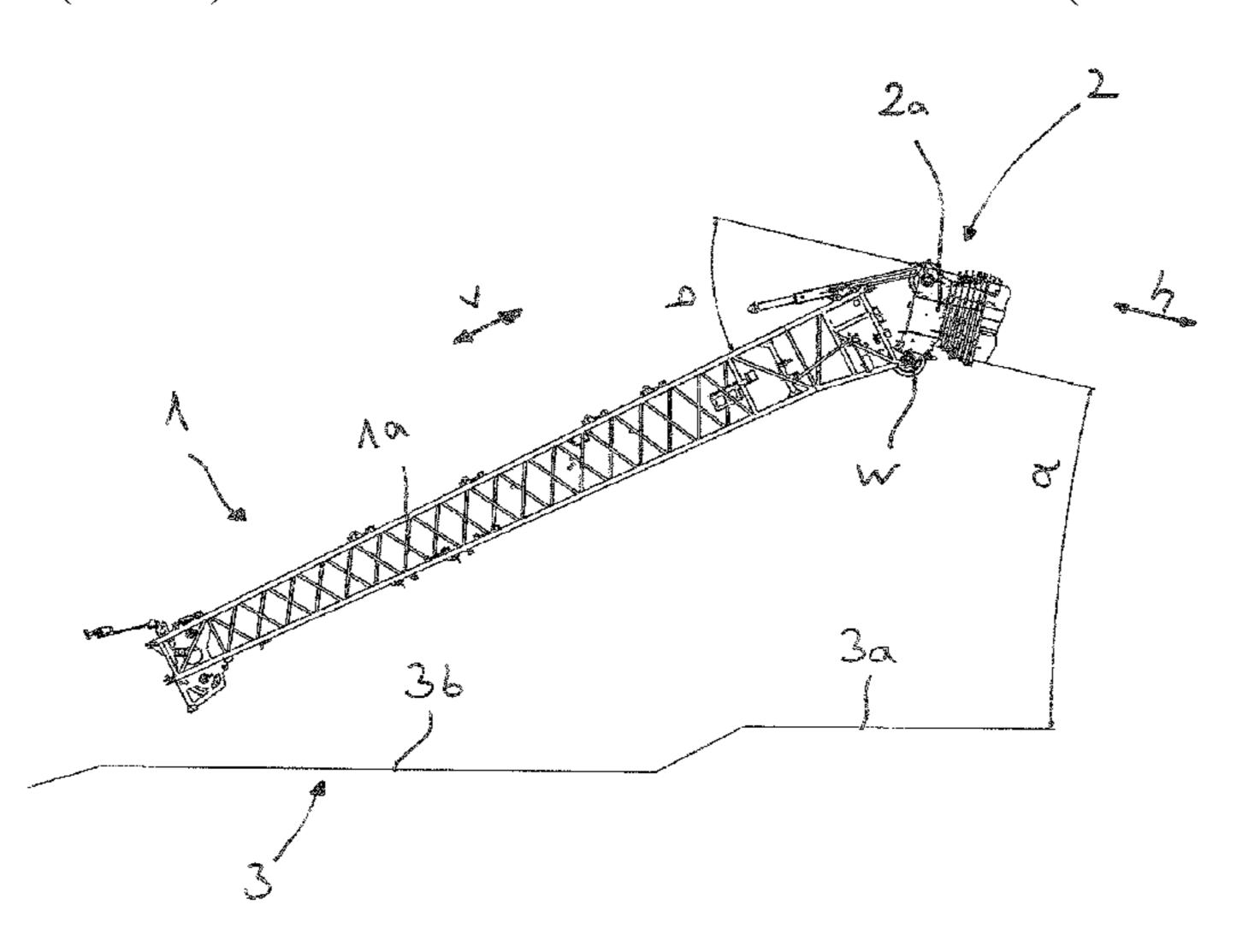
angling angle being delimited by an adjustable angling plate, and the angling plate engaging with the foot of the main jib extension and the main jib head. The angle drive may be a component of an angling plate in the form of a combiangling plate.
