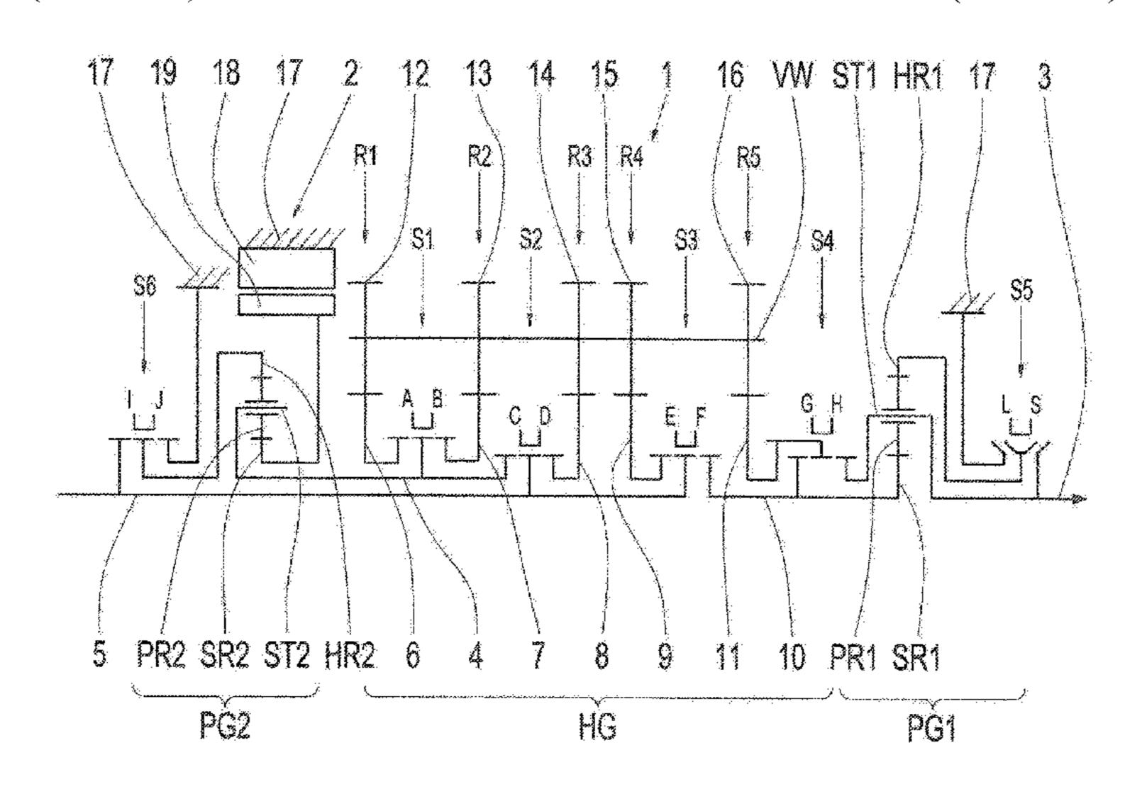
the main transmission (HG). The main transmission (HG) comprises first (R1), second (R2), third (R3), fourth (R4) and fifth gear planes (R5) and first (S1), second (S2), third (S3) and fourth shift elements (S4). Synchronization of the countershaft speed to a target speed, in direct gear, is performed via speed control of the electric machine (2).
