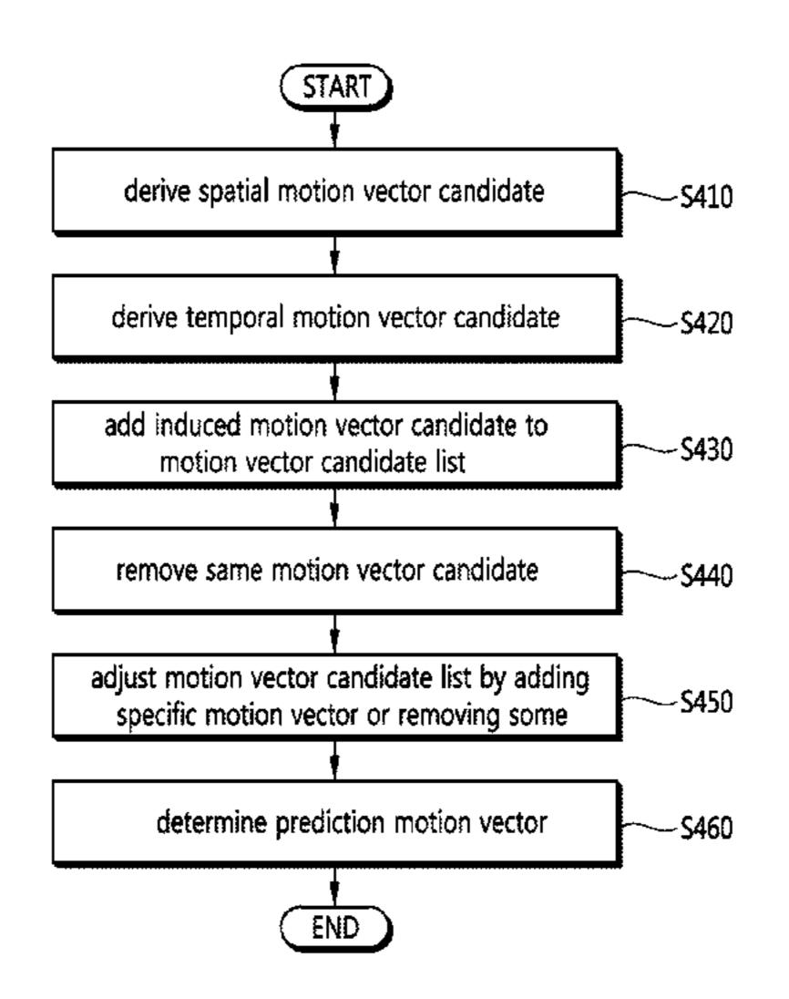
motion vector of the prediction block is determined on the basis of the adjusted motion vector candidate list. Accordingly, the complexity of arithmetic operations is reduced during encoding/decoding of an image.
