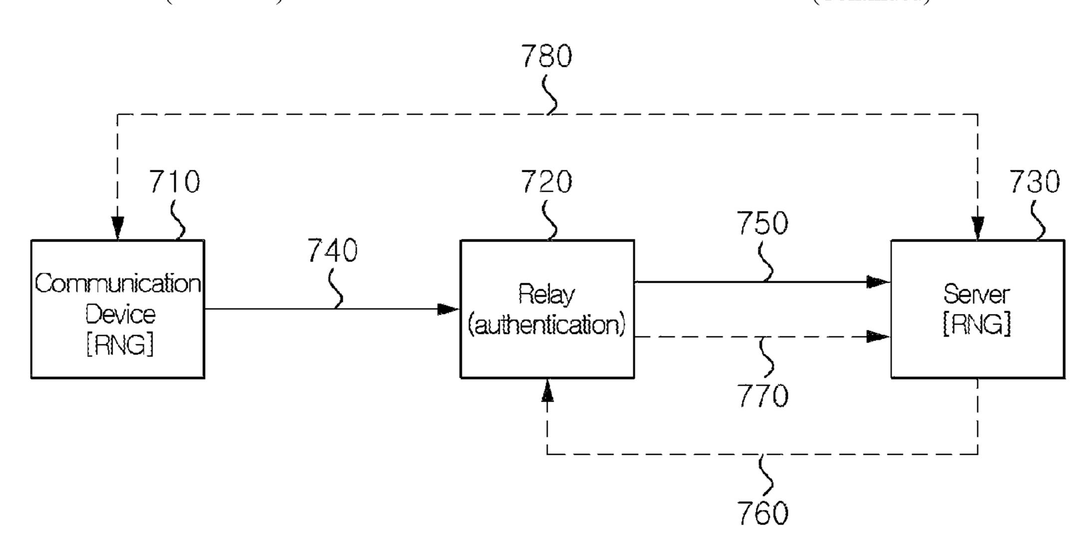
from a communication device pass through the second quantum filter of the relay device or a reception side, and the optical transmission unit transfers the series of second quantum signals to a server.
