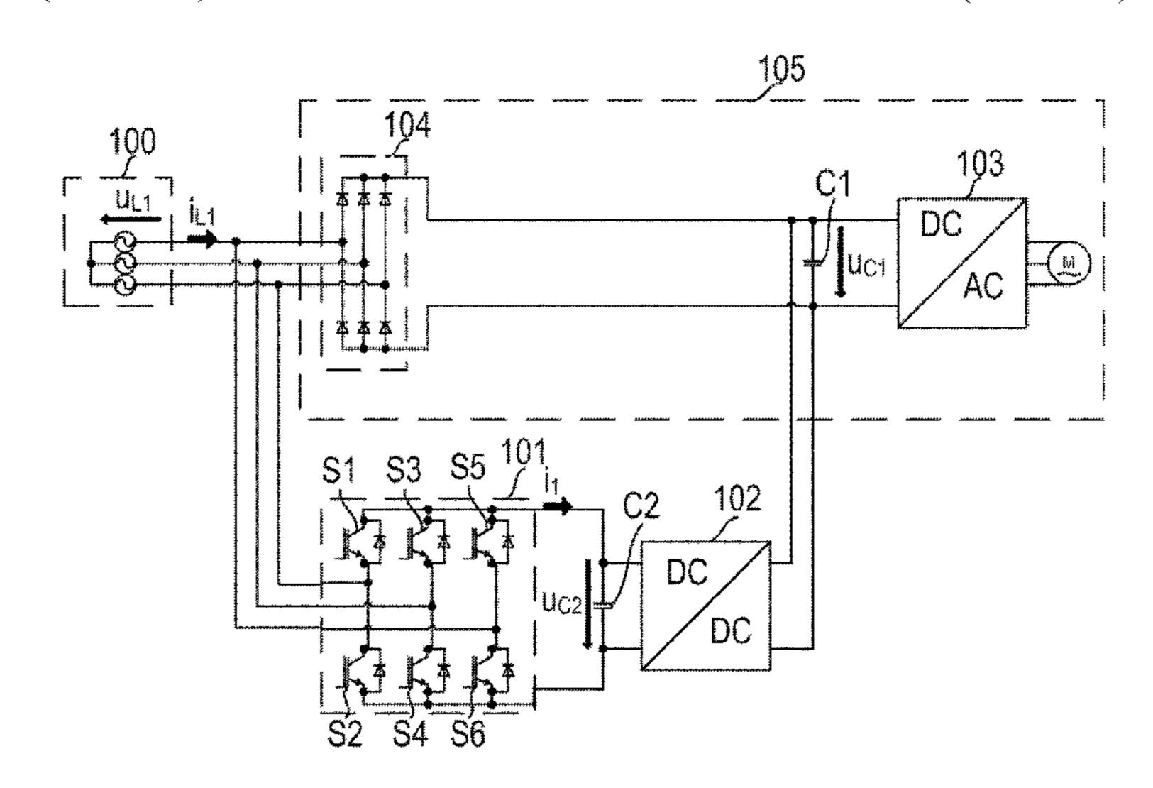
supplied to the control unit. The control unit supplies to the DC/DC transformer control signals such that the voltage supplied by the DC/DC transformer to the regenerative power inverter, the acquired current is able to be controlled, in particular controls, to a setpoint-value characteristic.
