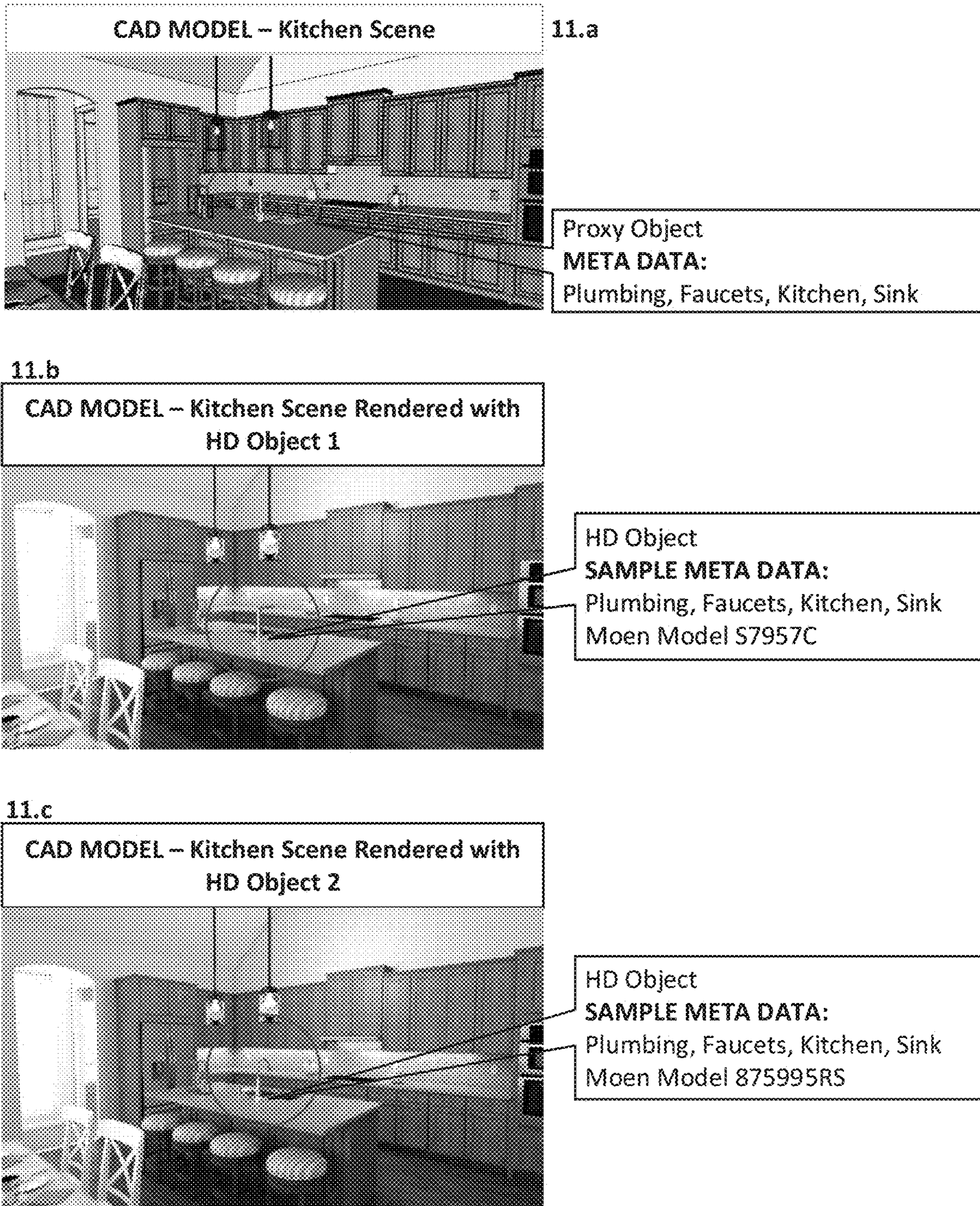
Figure 11: Swapping Object in CAD Model Example
