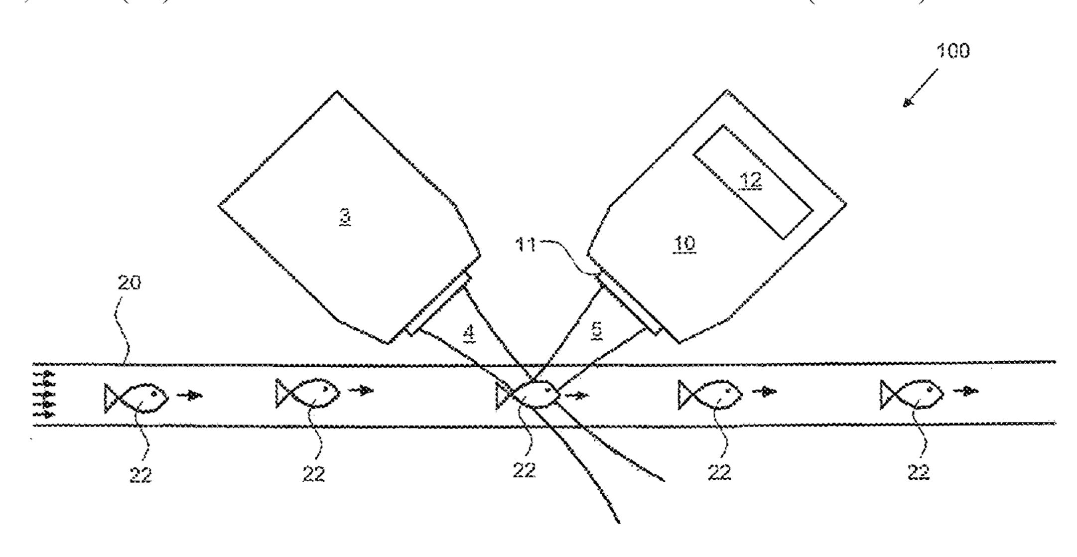
ing to the invention, the microscope is characterized in that the imaging means comprise a detection lens having a stationary front optics and movable focusing optics, wherein the focusing optics is arranged behind the front optics and in front of an intermediate image plane, and can be adjusted for the height adjustment of a detection plane. The invention further relates to a corresponding microscopy method.
