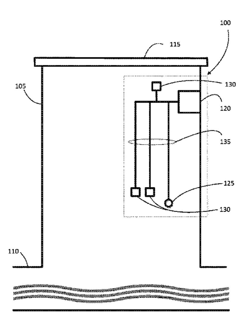
to supply power to the at least one sensor in response to receiving an output signal from the at least one threshold level indicator indicative of the fluid level having exceeded the threshold fluid level.
