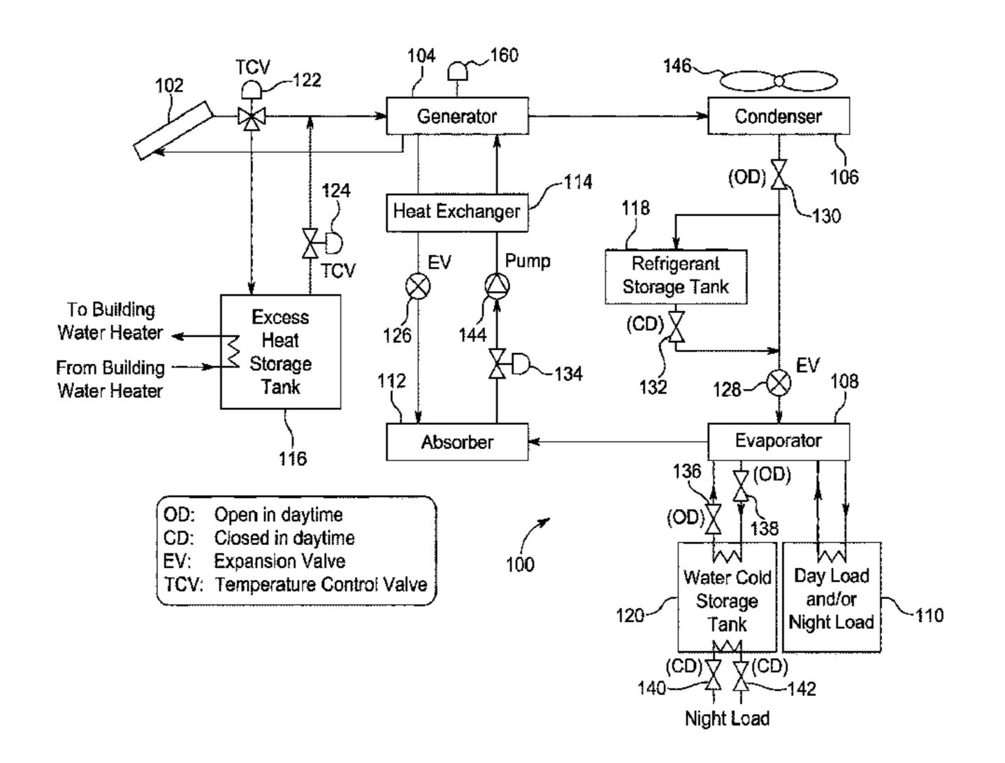
or a closed mode in response to a controller signal indicating a presence or an absence of a set point of a solid absorbent content in the dilute absorbent-refrigerant solution of the generator.
