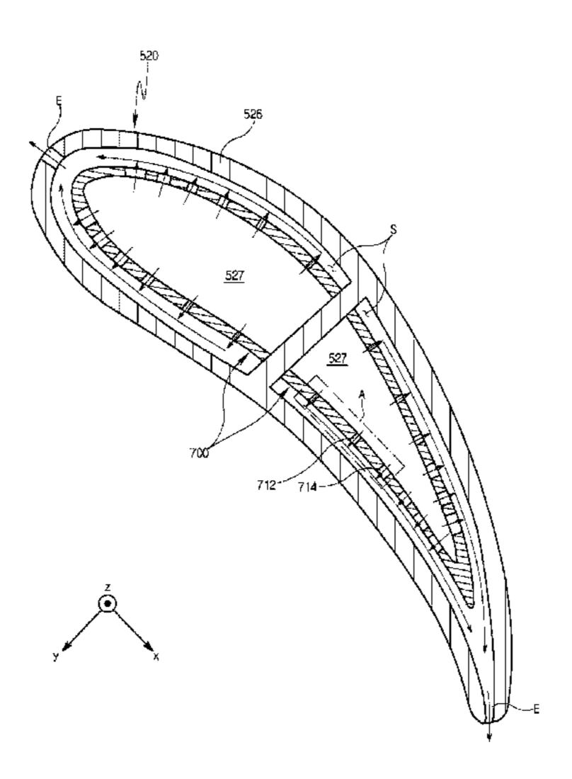
turbine vane that is cooled by cooling fluid ejected from the impingement plate.
