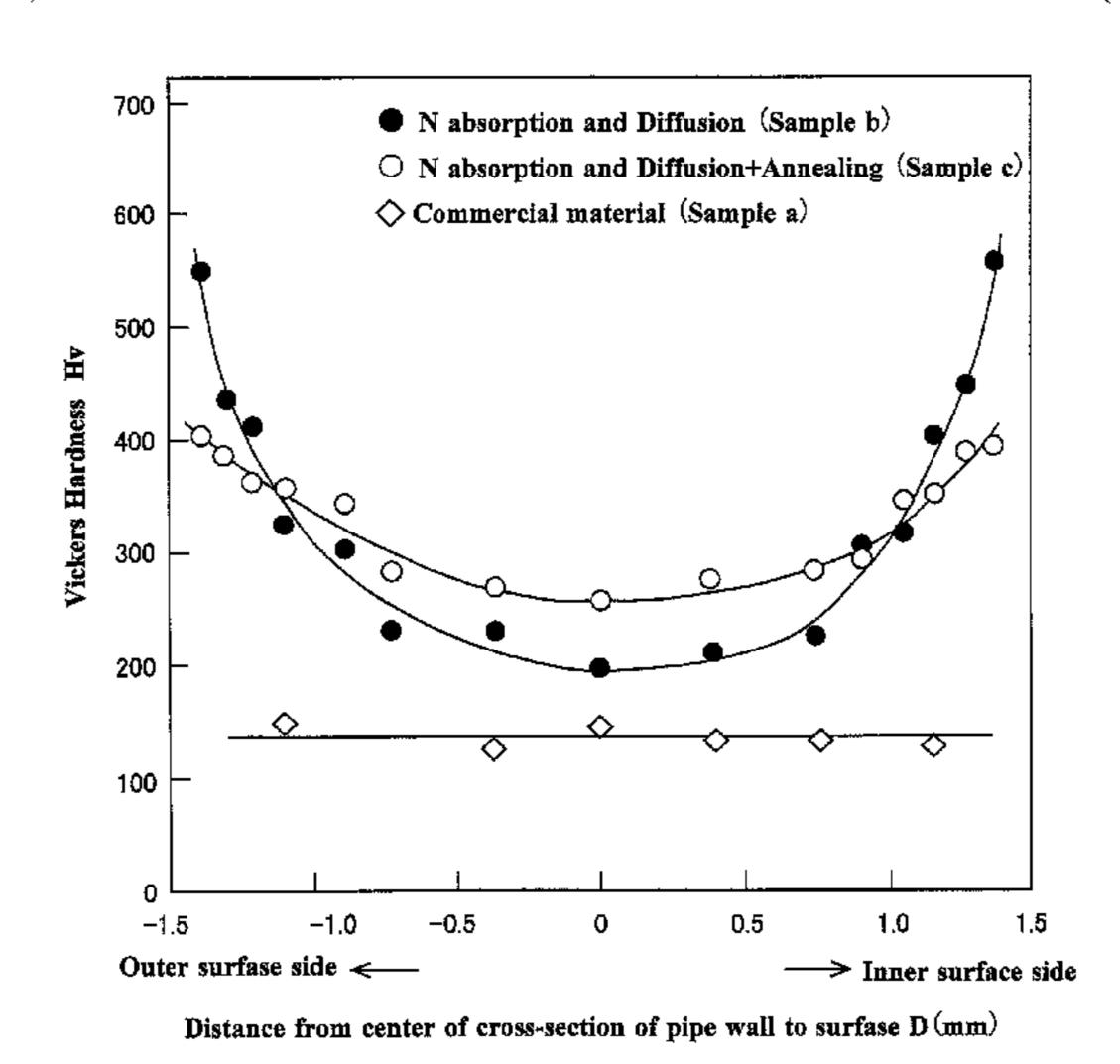
of conventional austenite stainless steel pipe materials and enhancing characteristic of anti-hydrogen gas embrittlement (anti-HGE) so as to be suitable for use in a high pressure hydrogen tank utilized in hydrogen cell vehicle (FCV) and a liquid hydrogen tank.
