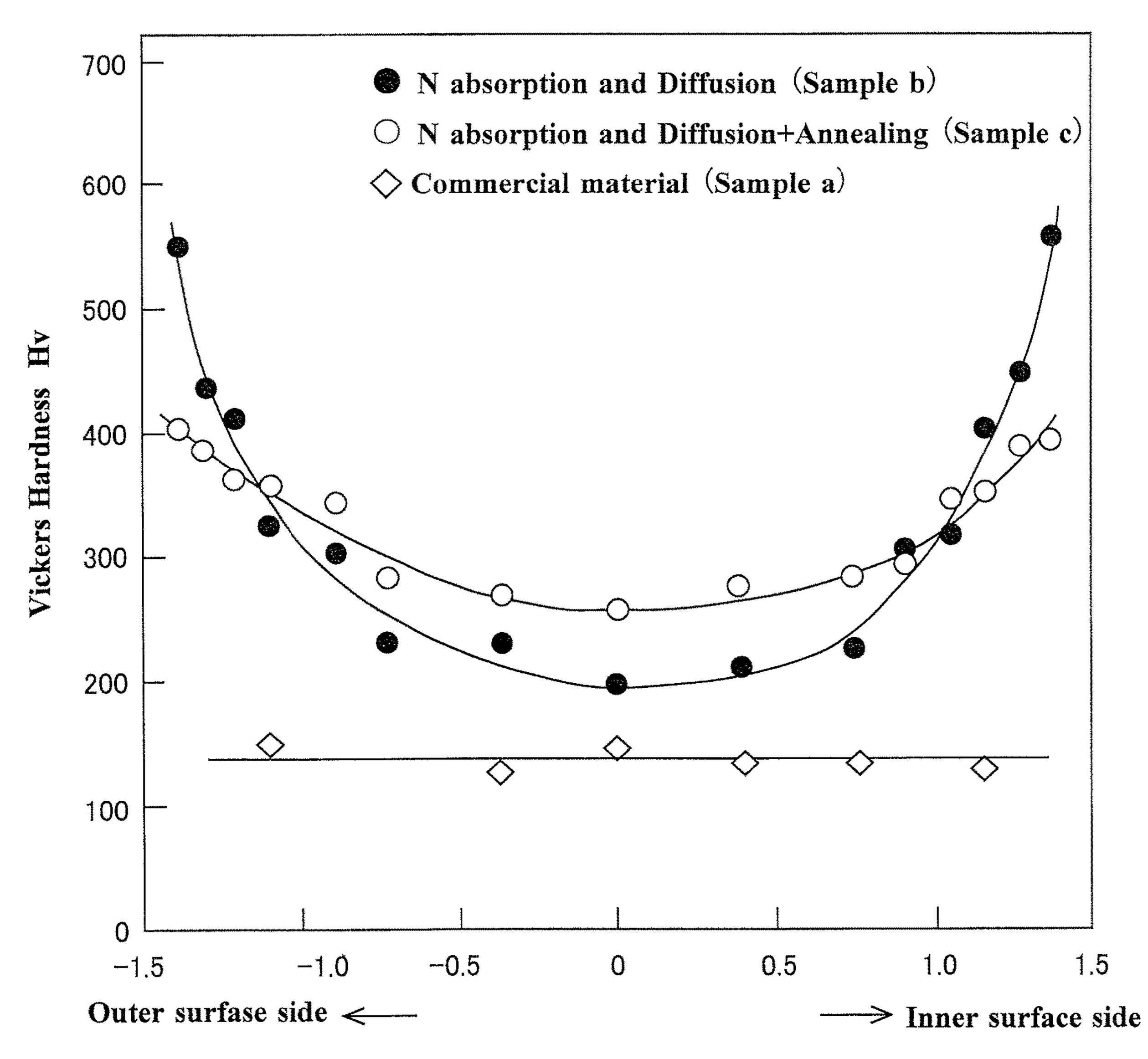
Distance from center of cross-section of pipe wall to surfase D (mm)
