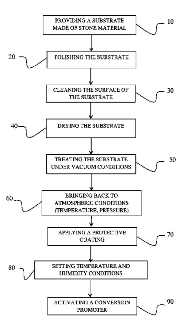
pressure, it is possible to apply and effectively adhere the protective coating to the surface of the stone material.
