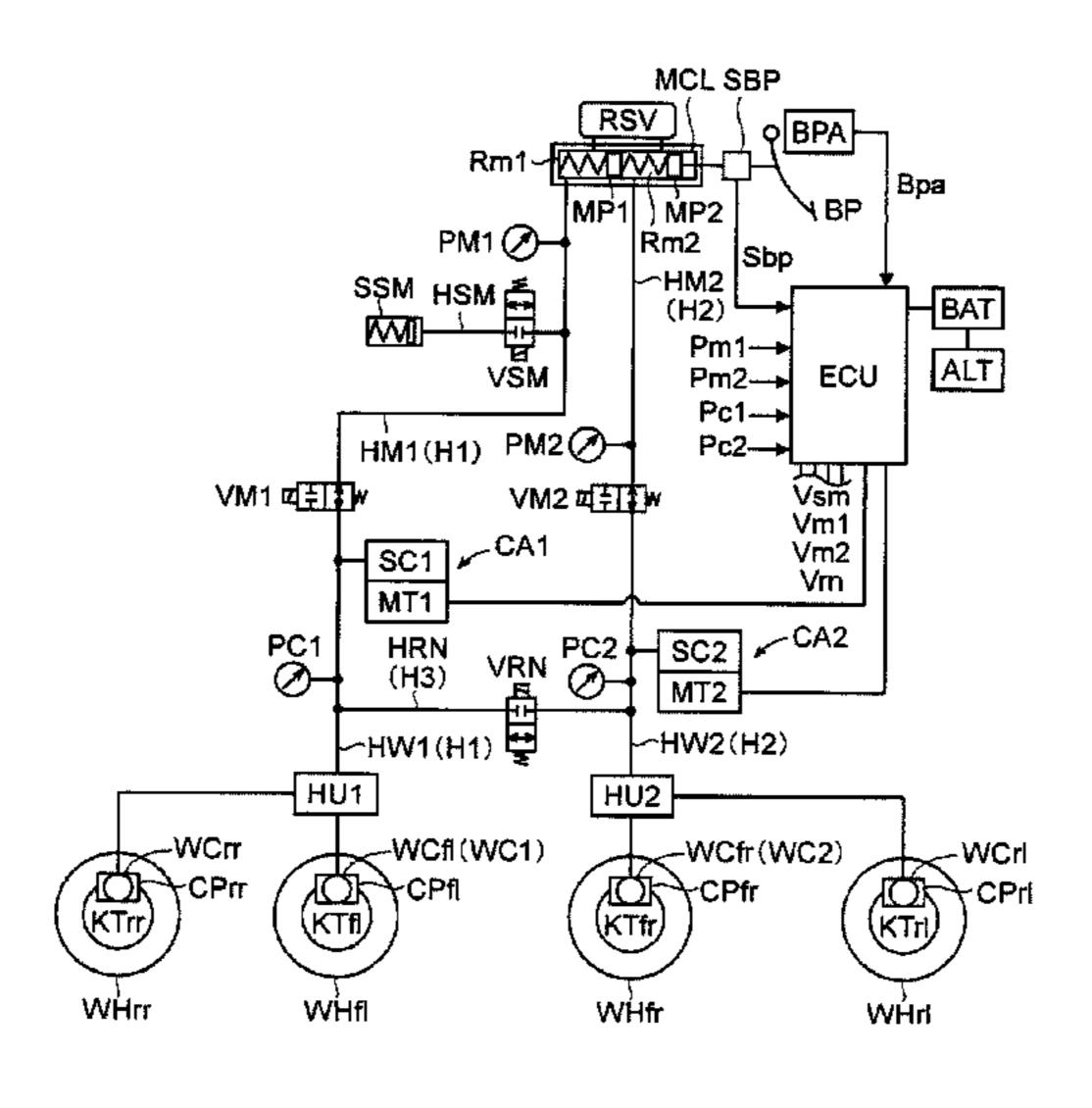
the control means puts the opening/closing means in a connected state, puts the first electric motor in an electricity-supplied state, and puts the second electric motor in a non-electricity-supplied state.
