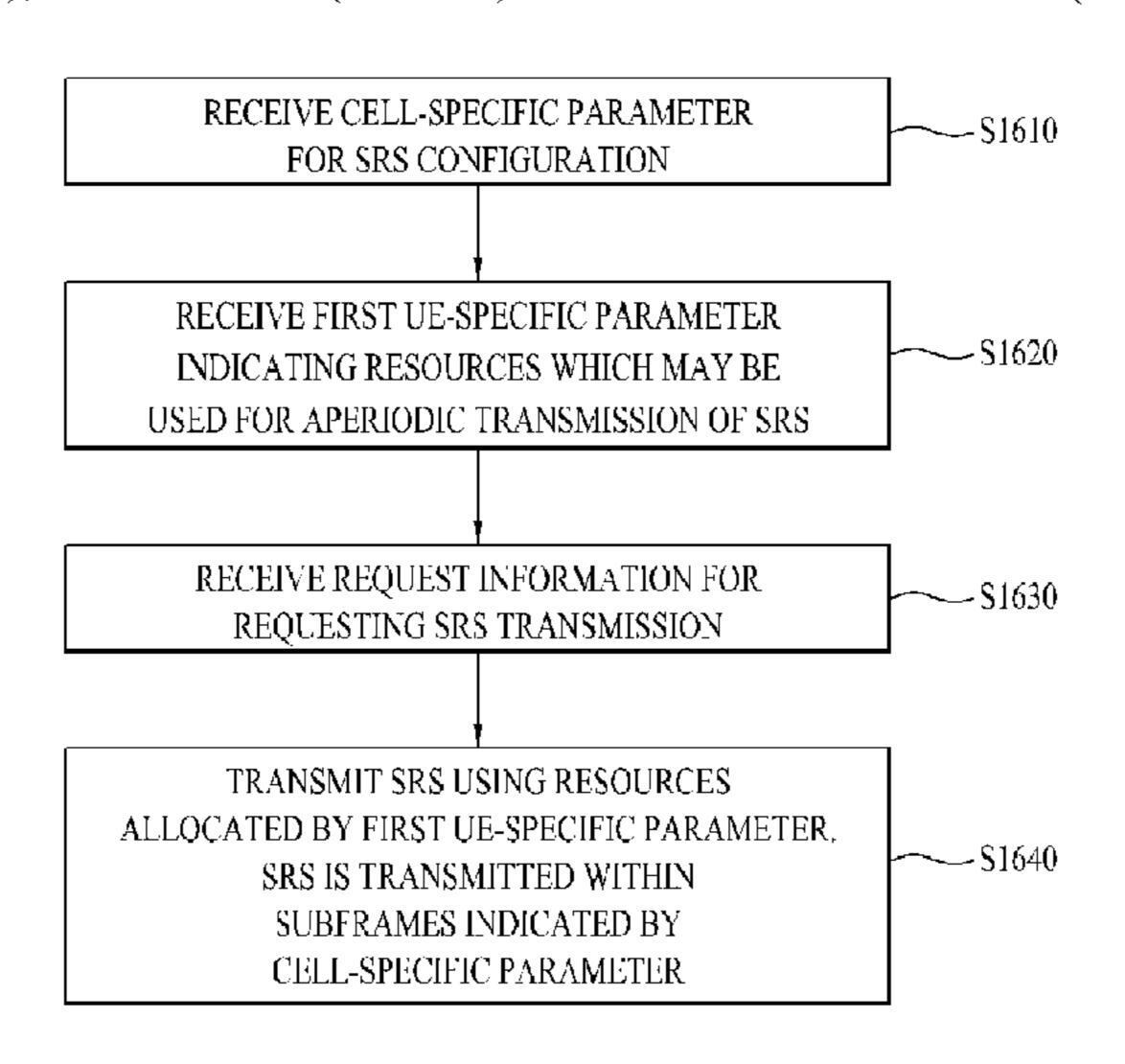
tion of request information for requesting a transmission of the SRS, and wherein, if the indicator indicates that the periodic SRS transmission is performed, the SRS is periodically transmitted in the configured subframe.
