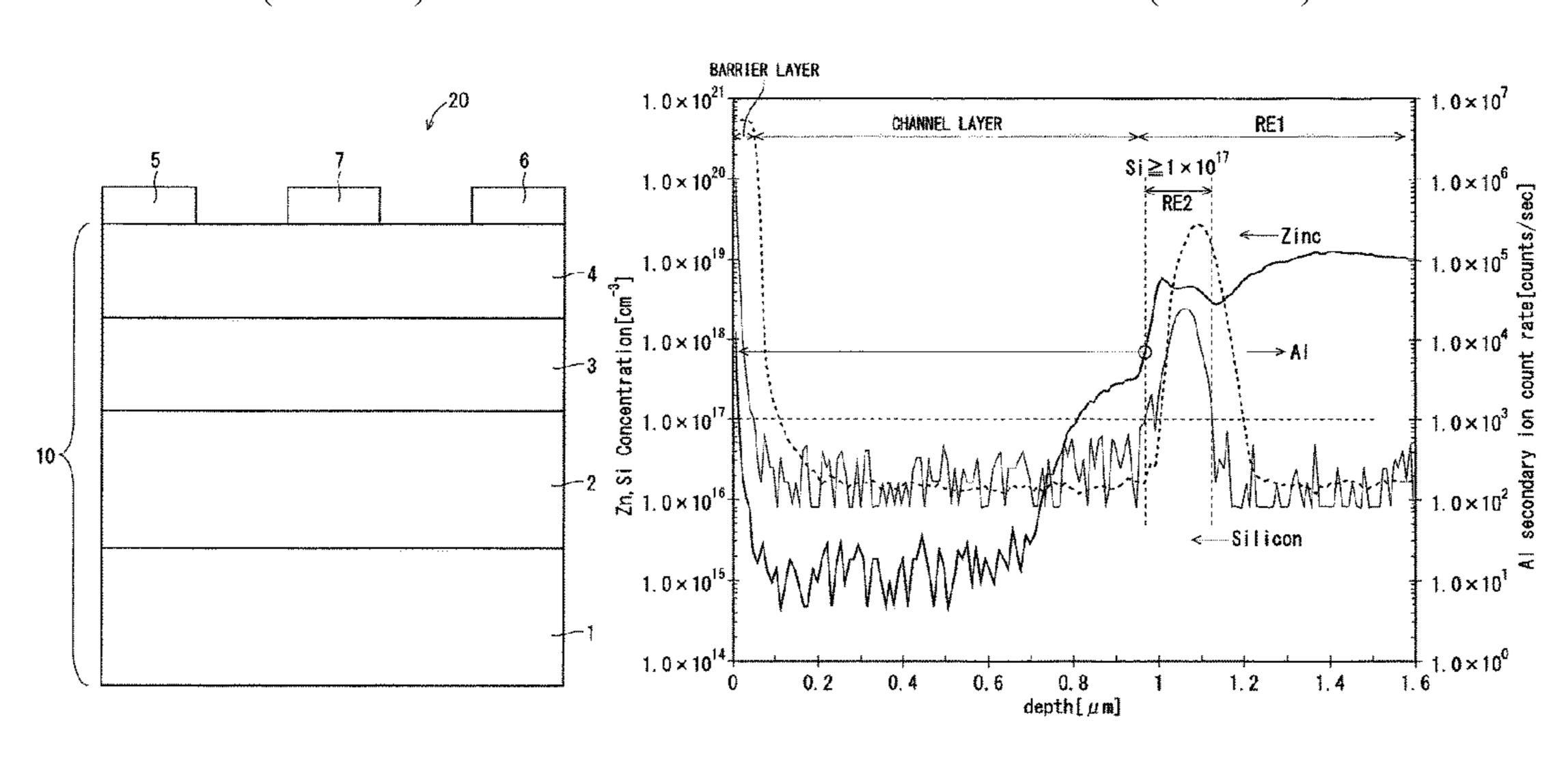
Si at a concentration of  $1 \times 10^{17}$  cm<sup>-3</sup> or more, and a minimum value of a concentration of Zn in the second region is  $1 \times 10^{17}$  cm<sup>-3</sup>.
