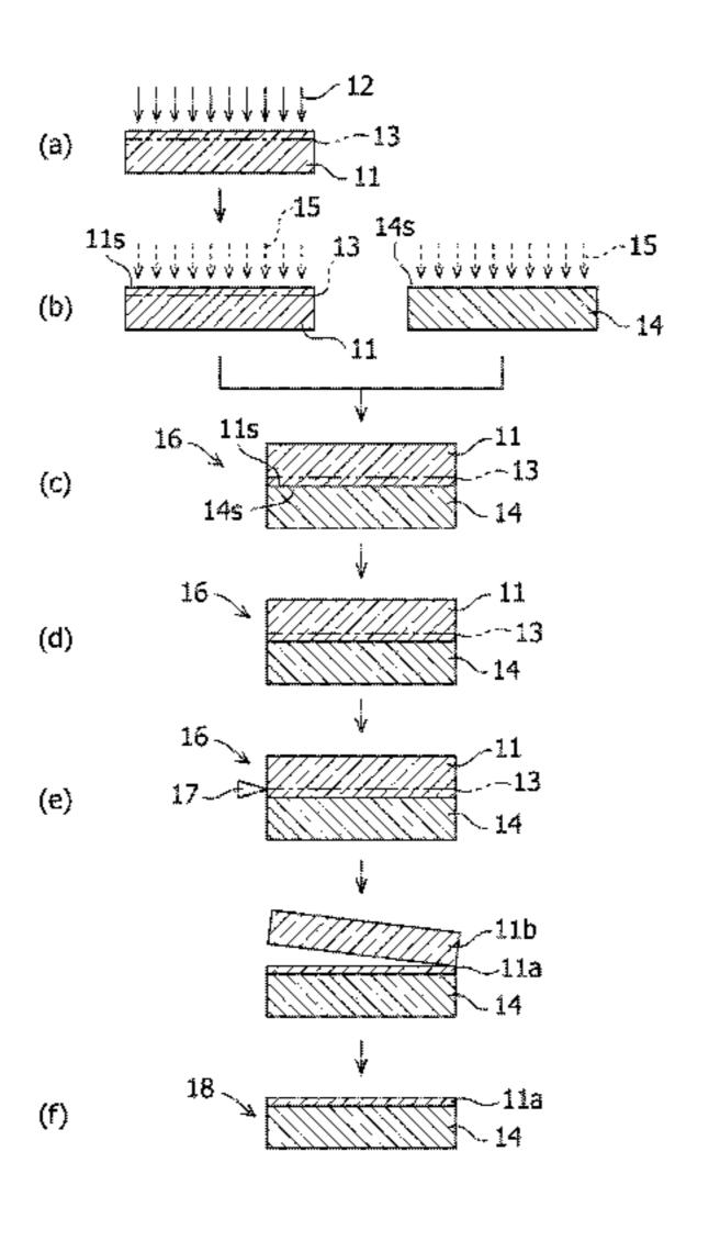
layer, and a step of subjecting the support wafer having the transferred oxide single crystal thin film to a second heat treatment at 250° C. to 600° C. to yield a composite wafer.
