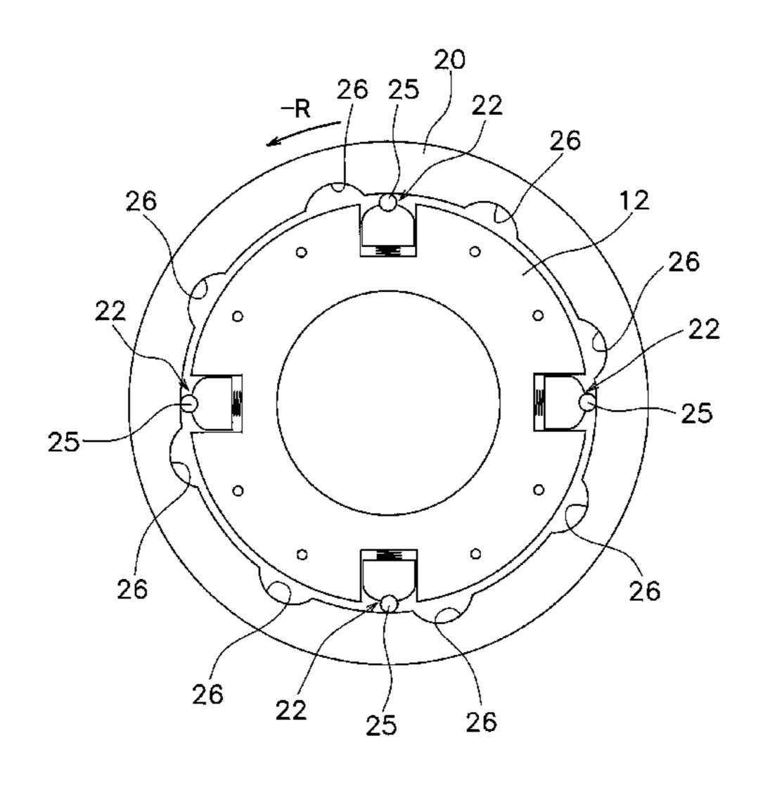
force directed to reduce the relative displacement. Additionally, when the torque fluctuations inputted to the rotor have a predetermined magnitude or greater, the cam mechanism makes the mass body freely rotate with respect to the rotor.
