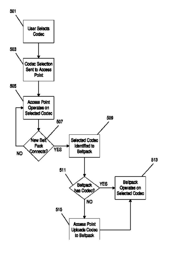
codec to the new intercom device and transmits communications with the intercom device—including, for example, audio stream data—using the selected codec.
