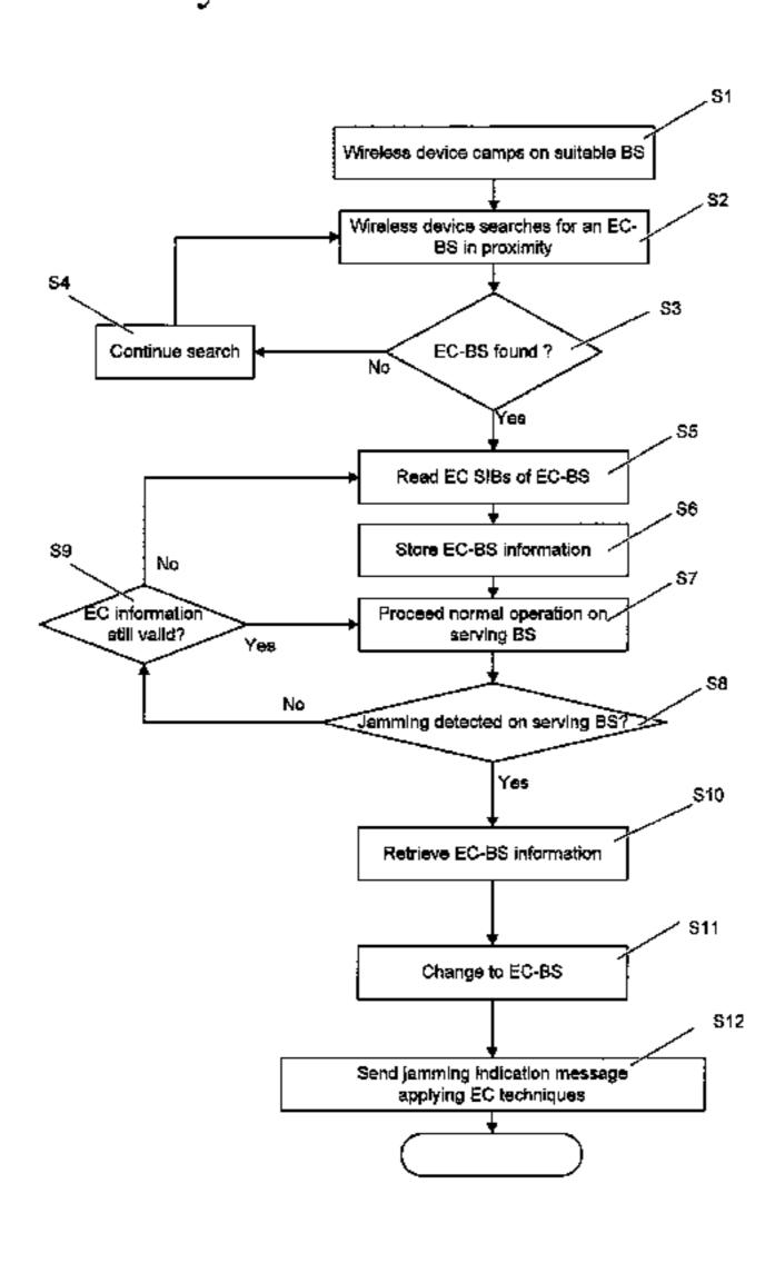
operation with said enhanced coverage base station in enhanced coverage mode, and sending a jamming indication message to a remote server accessible via the cellular network by means of said enhanced coverage base station.
