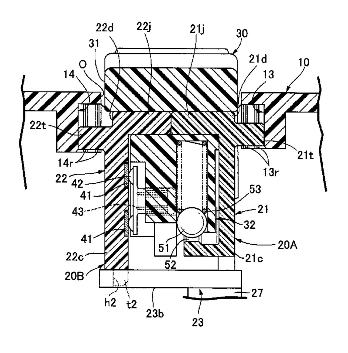
of the pair of shaft portions respectively. Such arrangement prevents switch malfunctioning, and restrains deformation of the side wall parts.
