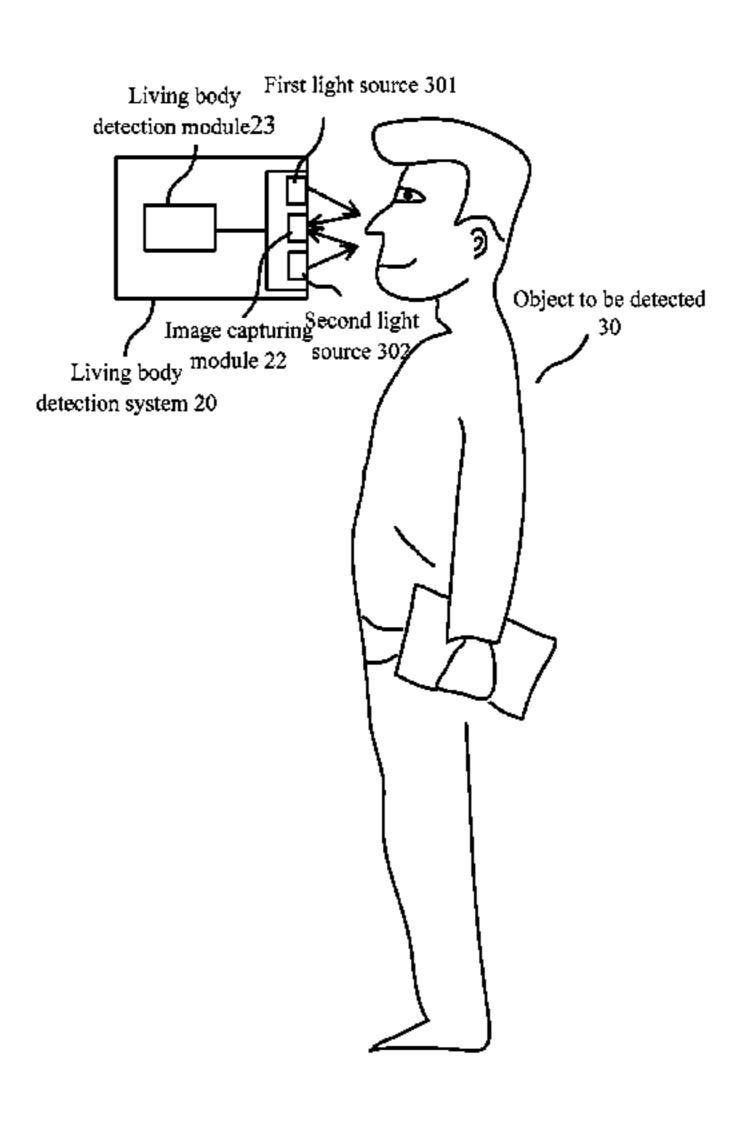
the object to be detected is a living body if the detection value is greater than a pre-determined threshold value.
