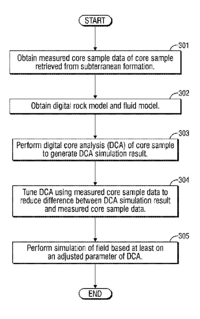
generate a DCA simulation result and the DCA is tuned using the measured core sample data to reduce a difference between the DCA simulation result and the measured core sample data. The tuning is performed by adjusting, in response to the difference exceeding a pre-determined limit, a parameter of the DCA to generate an adjusted parameter and further performing the DCA to reduce the difference.
