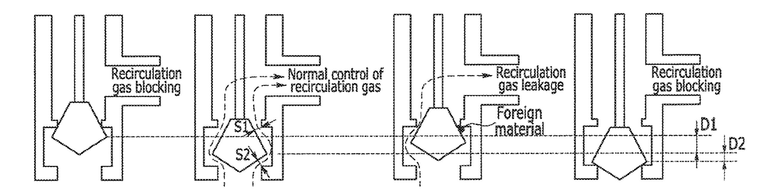
Normal blocking position Maximum open position Abnormal blocking position
