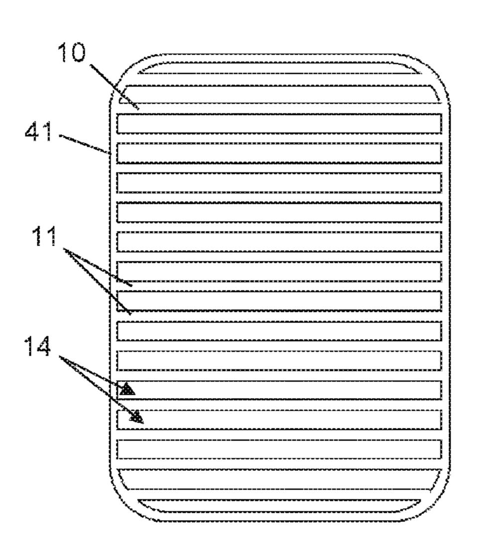
design of the assembly (1) in which anti-biofouling of the entire grating (10) may be guaranteed.
