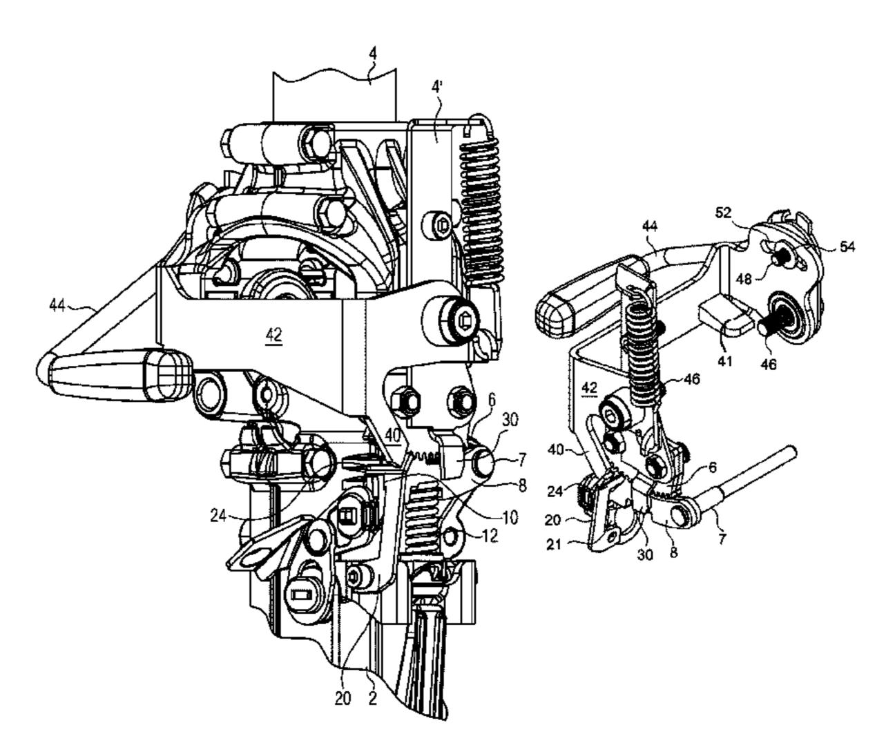
is moved out of engagement with the tooth hook (8) so that the tooth hook is biased back to the engaged position with the tooth segment (6).
