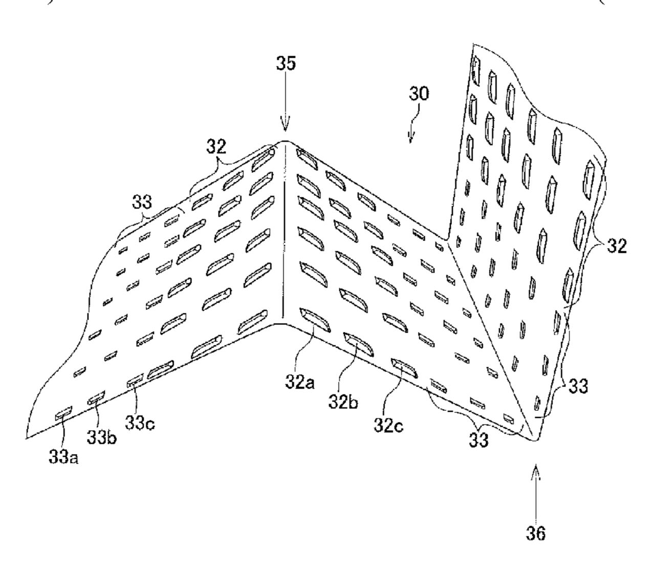
side. In the pleated state, the downwind-surface interval maintaining structure maintains an interval between facing downwind surfaces at least at a portion on an air-flow downstream side of the center of the air-filtering medium in the direction of airflow. In the pleated state, the upwind-surface interval maintaining member maintains an interval between facing upwind surfaces at least at a portion on the downstream side of the center of the air-filtering medium in the direction of airflow.
