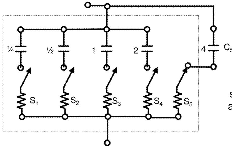
Uses external high Q cap to allow the switch to be smaller and still maintain the Q of the total Cap
