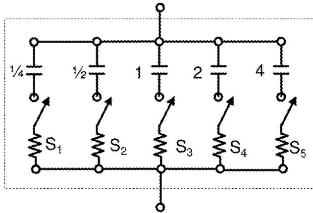
Reduce size of  $S_5$  to make Q only good in low band since circuits usually need less capacitance in high band.
