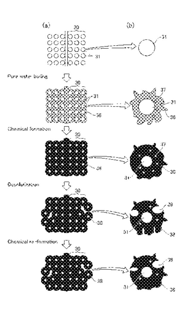
step, a phosphoric acid immersion step of immersing the aluminum electrode in an aqueous solution containing phosphate ions is carried out one or more times in the course of raising a film withstand voltage to a chemical formation voltage.
